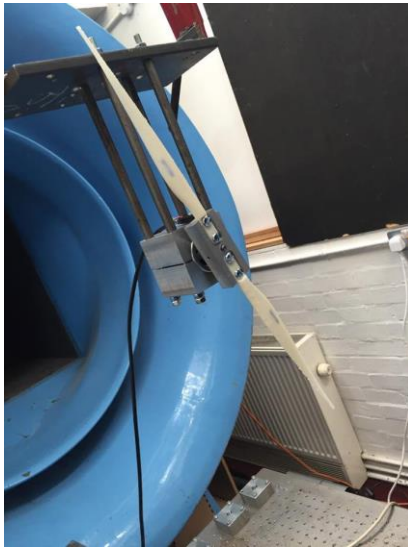
Figure 45 - Wind turbine blades (13g pair) mounted on the motor for wind tunnel testing
