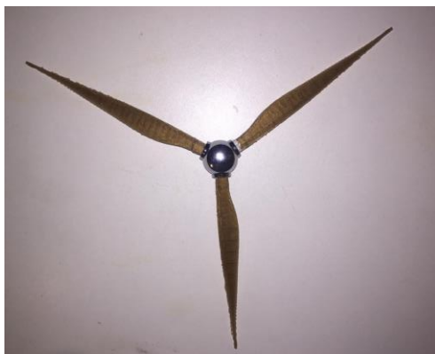
Figure 50 - Assembled wind turbine blades attached to hub
